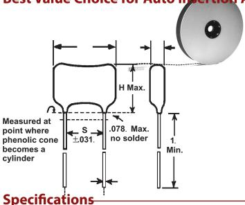
Type CDA15 is designed especially for auto-insertion and is the best value choice for tape and reel and ammo-pack feed systems. CDA15 is used in commercial and industrial applications requiring high stability, high Q and close capacitance tolerances. Type CDA15 is ideal for tuned circuits, delay lines and filter circuits.
